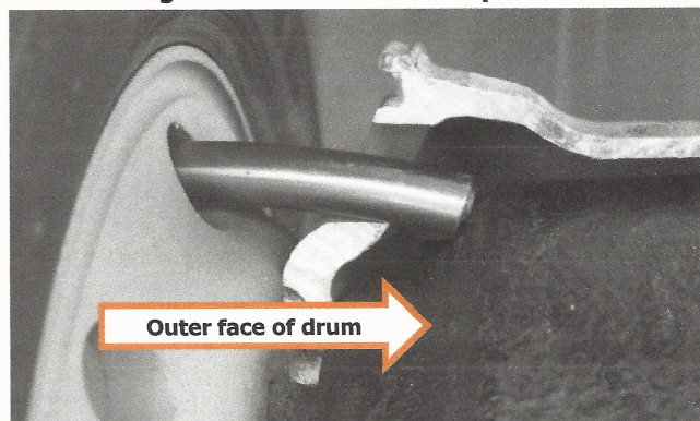
Fig. 4 - Protective rubber sleeve in place
